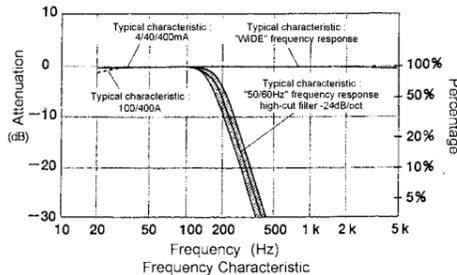
Recently there has been increased use of power through inverters, switching regulators, etc. When the high frequency noise from such appliances leaks or flows into the ground through capacitors not filtering completely, the earth leakage breaker may trip even though there is no "actual" leakage. In such a case, the instrument do not give leakage current reading if "50/60Hz" frequency response is selected.
