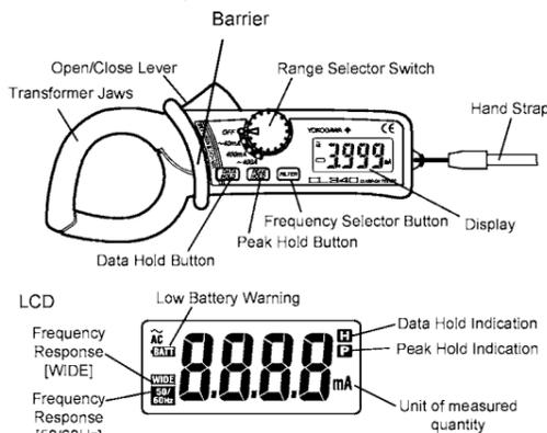
**Barrier** : It is a part providing protection against electrical shock and ensuring the minimum required air and creep age distances.
