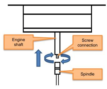
Note: Be careful when attaching the spindle to prevent damage to the spindle and shaft.
