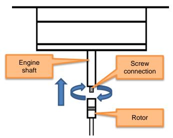
Note: Be careful when attaching the rotor to prevent damage to the rotor and shaft.
