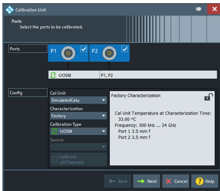
Figure 8-11: Calibration Unit wizard, step 1: Ports
