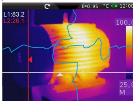
Fig. 26: Display of Measuring lines
