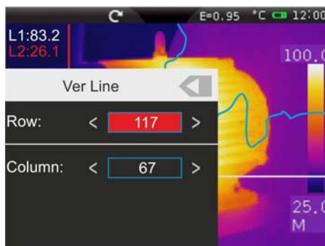
Fig. 27: Setting the position of the cursor of the Line
