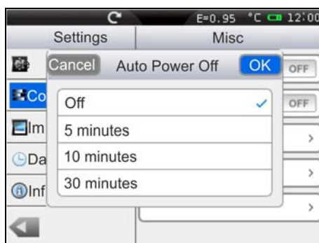
Fig. 16: Setting the instrument's auto power-off time
