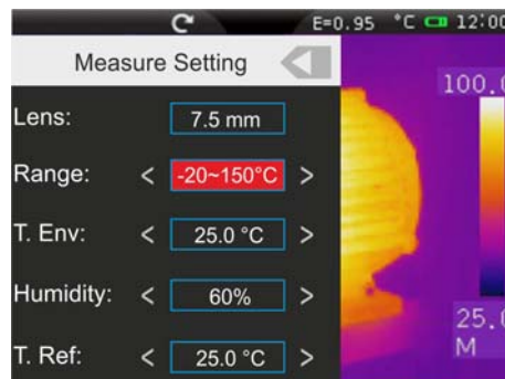
Fig. 39: Setting the general measuring parameters
