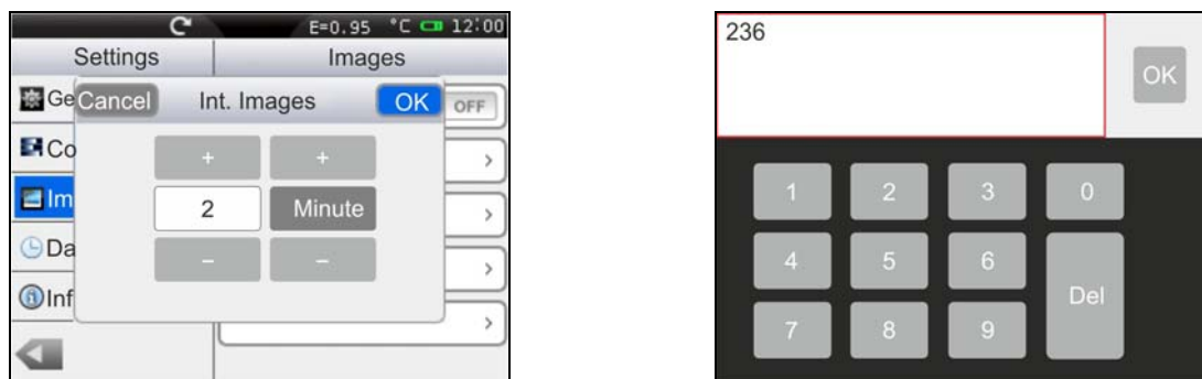
Fig. 18: Setting the image saving time
