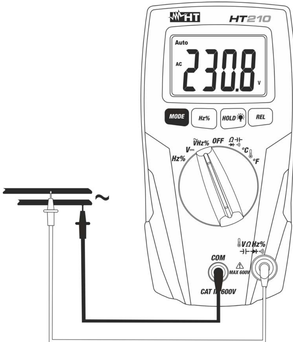
Fig. 3: Using the instrument for AC Voltage measurement
