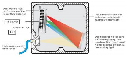
LMS-9000 used the Band pass-filter Wheel Correcting Technique, Spectrometer & Broadband-radiometer & photometer Combined Technique, and modified NIST stray light correction technology, the LMS-9000 spectroradiometer can realize ultra low stray light and super photometry linearity in overall dynamic range.
