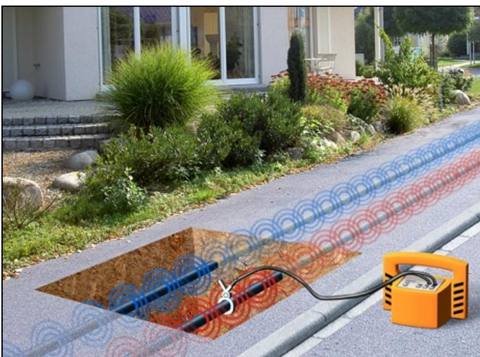
**Coupling via transmitter clamp** In doing so, it is **not** necessary to disconnect the cables
