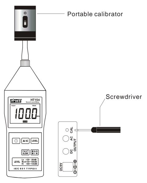
Fig. 4: Connection of meter to portable calibrator HT150
