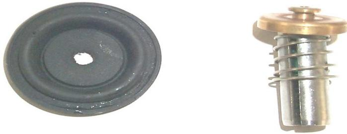
10) Inspect the rubber diaphragm to verify the defect/damage.
