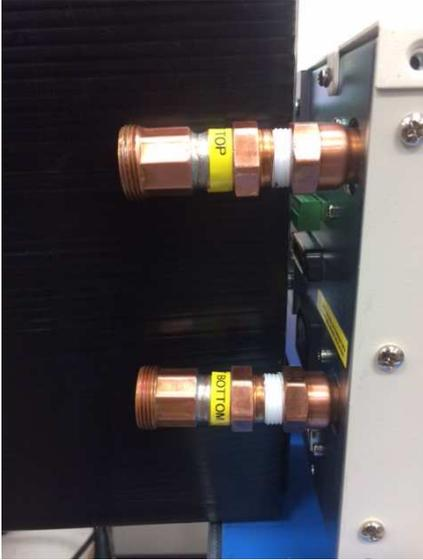
Locate the FLUID OUTLET distribution pipe. Install onto the interconnect pipes. Using one ranch fixed position on the interconnect pipes, and the other ranch torque carefully at the distribution pipe.
