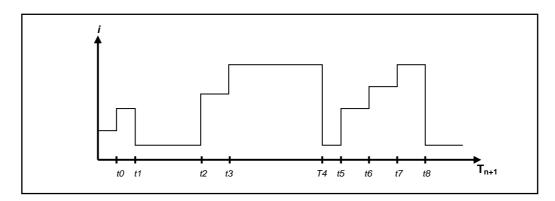
**STEP:** The Step mode will repeat the step cycle until the end of the dwell time without the need for a trigger signal. Once transient level is activated, the STEP mode will start as well.
