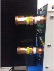
Locate the FLUID OUTLET distribution pipe. Install onto the interconnect pipes. Using one ranch fixed position on the interconnect pipes, and the other ranch torque
