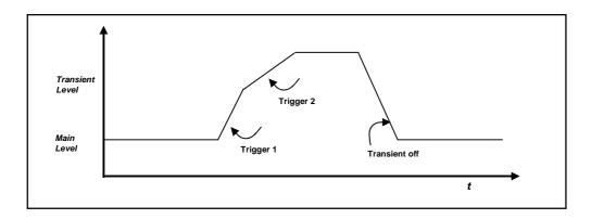
**Note:** All the operating modes can be programmed via the front panel or using GPIB/RS232/ETHERNET/USB Interfaces with the exception of TRIGGER operation, which is remotely controlled. In addition, each transient mode besides CONTINUOUS can be triggered through a negative edge triggered external TTL compatible signal. CONTINUOUS Transient Operation will start as soon as PULSE is activated, and can not be activated using a trigger signal.
