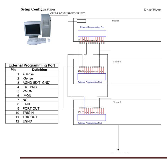
More devices can be paralleled by daisy chain the Trig\_Out of each unit to the Trig\_In of the other unit for digital control signal and by connecting the IMON of the Master unit to the EXT\_PRG of the Slave units for analog control signal. Be sure the signal return is different between digital signal (EGND) and analog signal (AGND). Connect the RY\_NO of each Slave unit to RI of Master unit for System Fault operation.
