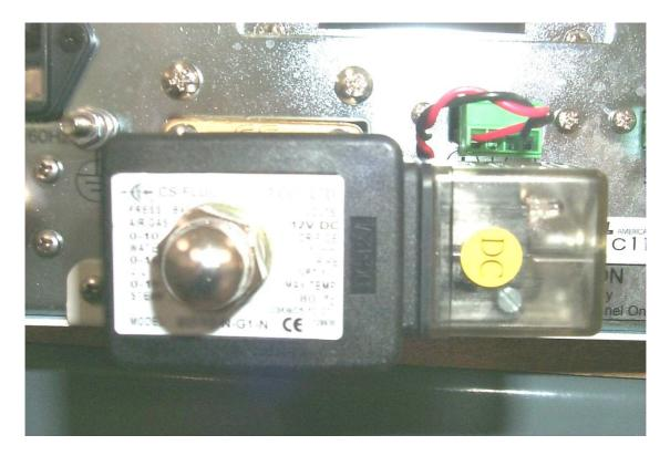
2) Unplug the  $12V_{\text{DC}}$  connector (4 pin), remove the hexagonal nut and take off the coil assembly.
