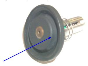
9) Separate the rubber diaphragm from the metal solenoid assembly.
