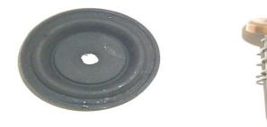
10) Inspect the rubber diaphragm to verify the defect/damage.
