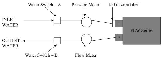
FIGURE 2.2 RECOMMENED PIPING AND COOLANT INSTALLATION
