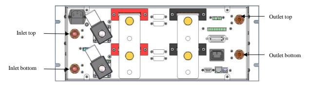
Use pipe thread sealant PTFE tape wrap approximately 3 to 4 times around each pipe male threads of each interconnect pipe, to ensure a tight seal and to prevent leak. Thoroughly clean the male and female thread and wrap the tap in the direction of the thread spiral. PTFE tape will not be included in the kit.
