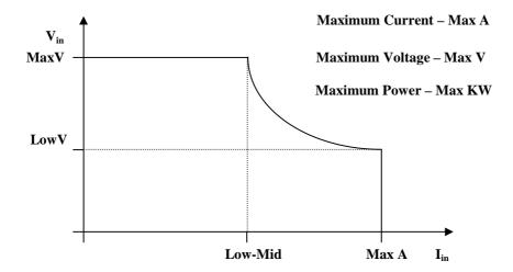
FIGURE 1.5 INPUT VOLTAGE/CURRENT/POWER RELATION DIAGRAM
