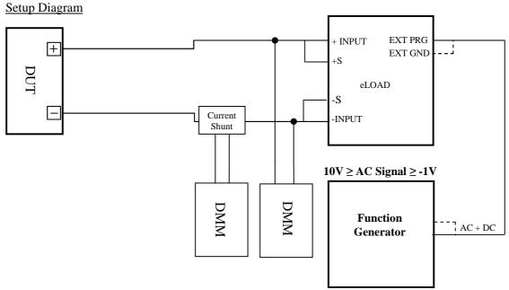
FIGURE 3.2 EXTERNAL PROGRAMMING SETUP
