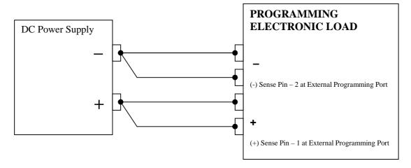
FIGURE 2.4 REMOTE SENSE CONFIGURATIONS
