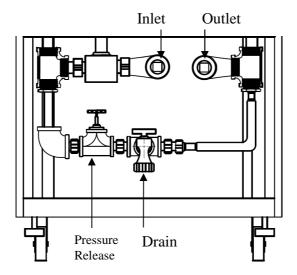
For PLW models **greater than** 4U height, unit will be ship in a cabinet with a pre-installed manifold system. Rear Panel diagram above illustrates positions of the cooling water **inlet** and **outlet** pipe as well as the **drain faucet** and **pressure release faucet**. Before filling the Load Bank with water, carefully read the following paragraphs for correct flow rate, water flow direction, and water pressure.
