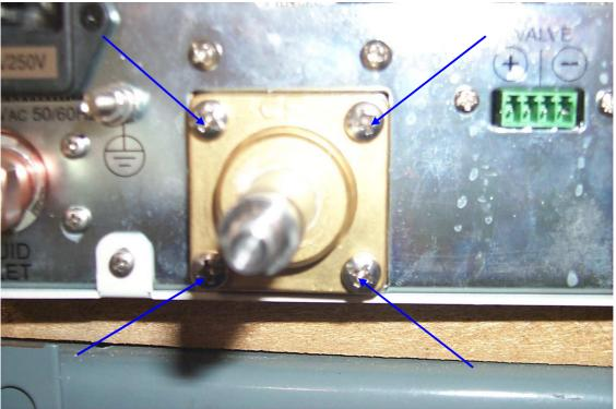
7) Place the coil assembly over the solenoid and re-bolt it tightly.
