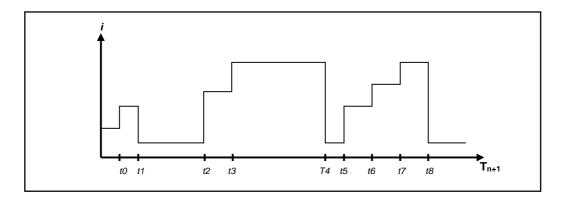
**STEP:** The Step mode will repeat the step cycle until the end of the dwell time without the need for a trigger signal. Once transient level is activated, the STEP mode will start as well.
