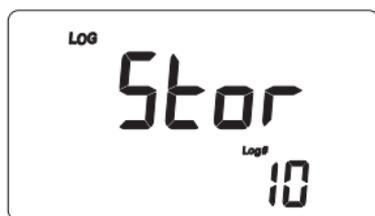
By pressing the STORE key a complete set of information is memorized: date, time, EC, TDS and temperature readings.
