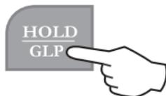
**Note:** Press HOLD key again to escape without deleting data. When scrolling through stored data, if a deleted sample is selected, the meter will display the "nuLL" message.
