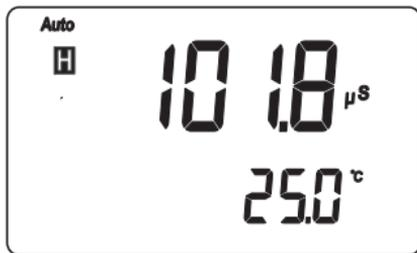
Press the HOLD key again to return the normal measurement mode.
