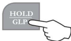
The "Auto" and "H" tags will blink on the LCD until the reading is stabilized.
