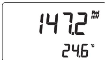
**Note:** The displayed relative mV reading is the difference between the current mV input value and the relative mV offset established in the relative mV calibration.
