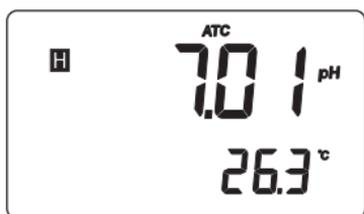
Press the HOLD key again to return the normal measurement mode.
