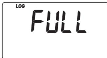
In this case, it is necessary to delete the last sample or all logged data to proceed.
