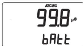
When the battery level is too low to ensure reliable readings, the meter automatically turns off.
