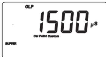
If the cell constant was changed after calibration (through the “CELL” setup item), this information is not displayed. If RANGE (or NEXT) is pressed while the last parameter is displayed, the meter returns to measurement mode.
