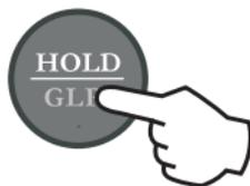
The "Auto" and "H" tags will blink on the LCD until the reading is stabilized.
