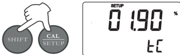
Select the desired setup item using the arrow keys, then press CFM to select and edit the setup item. The current value of the selected item starts blinking (if the parameter can be modified).
