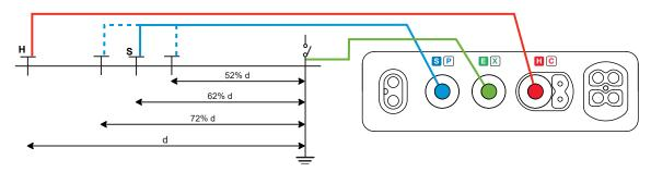
The 3 measurement results must be the same to within a few percent. If this is the case, the measurement is valid. If not, it is because the S rod is in the zone of influence of the earth electrode.
