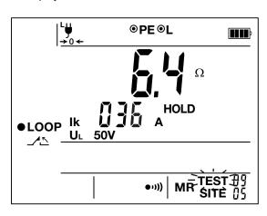
Pressing the ▶ key causes the SITE symbol to blink. You can change the site number using the ▲ key.
