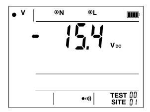
In the case of a live measurement (LOOP or RCD), the instrument shows where the phase should be on the outlet using the symbol. If the phase is on the wrong side, the symbol blinks to indicate that the tripod cable must be reversed.
