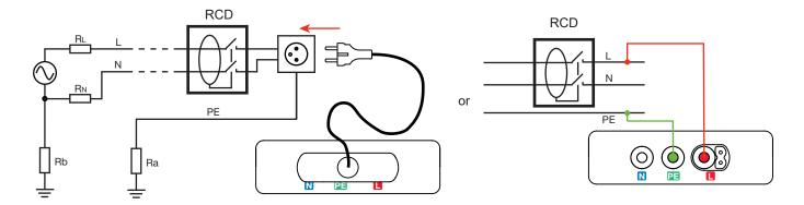
The instrument first of all checks that the voltage between the L and PE terminals is correct. If it is, the symbol lights steadily. If not, the symbol blinks and it is not possible to make a test.
