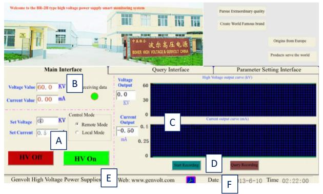
A: Set the control zone, first select the remote control mode, set the output voltage and current of the power supply, and then click to turn on the high voltage, the power supply can output the corresponding high voltage, current (The load should be appropriate, the power supply is constant power output, Excessive load will lead to low output voltage, too light load will make current less
