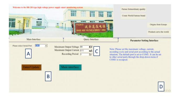
A: Used to set the communication serial port. The default is COM1.
