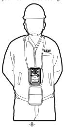
The safety voltage detector could be sensitive to static build-up and may become charged. In this case, this could trigger the alarm.
