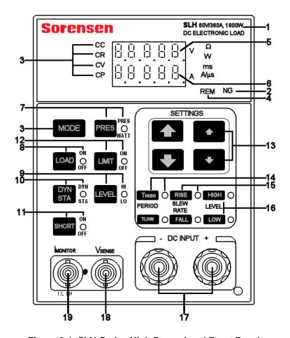
Figure 3-1 SLH-Series High Power Load Front Panel
