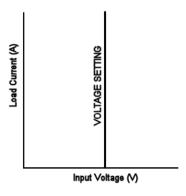
Figure 1-9 Constant Voltage (CV) Mode
