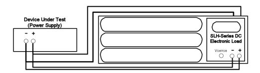
**Figure 4-1 Local Voltage Sense Connections**
