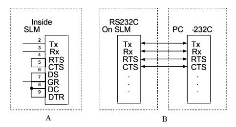
Figure 5-1 RS-232 Interface Diagram
