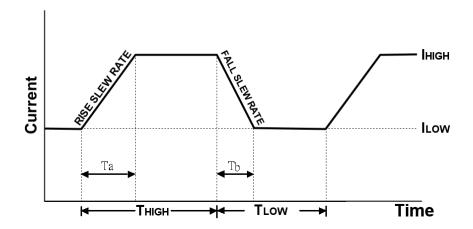
Figure 4-4 Dynamic Load Current with Independent Programmed Rise/Fall Slew Rate
