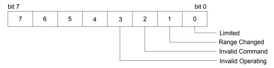
Figure 5-3 Error Status Byte Register
