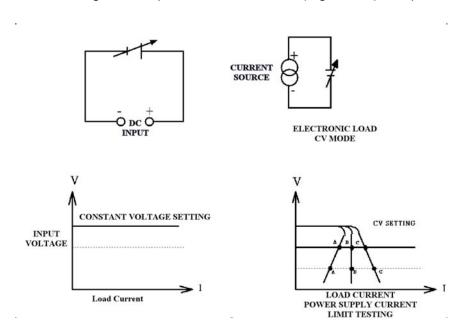
**Figure 4-5 Constant Voltage Mode Application**
