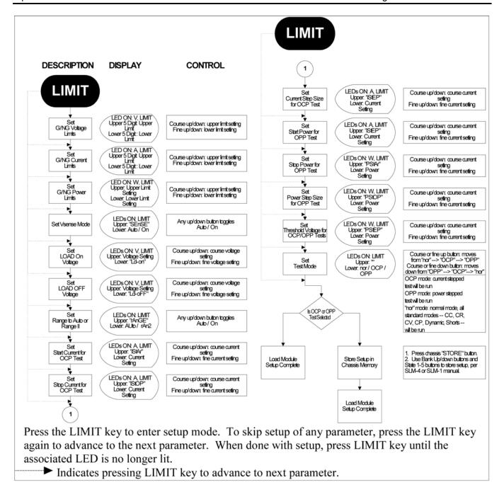
Figure 3-3 Flow Chart for Load Module General Setup Parameters and OCP and OPP Tests
