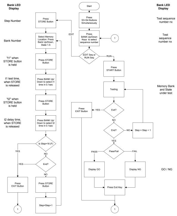
Figure 3-7 Auto Sequence Function Set-Up and Operation Flowchart
