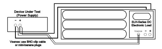
Figure 4-2 Remote Voltage Sense Connections
