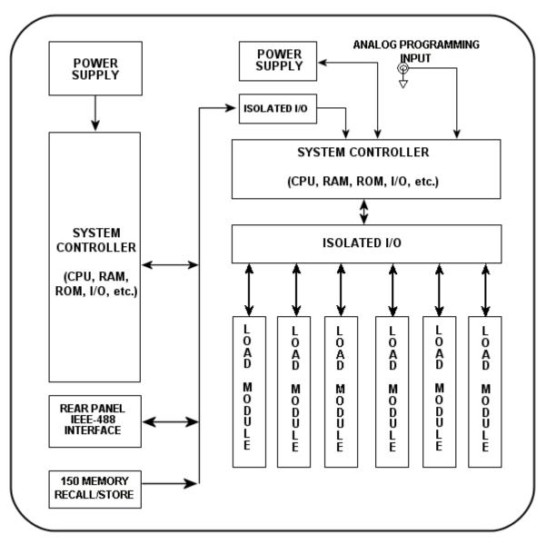
Figure 1-11 Block Diagram of SLH-Series Electronic Load
