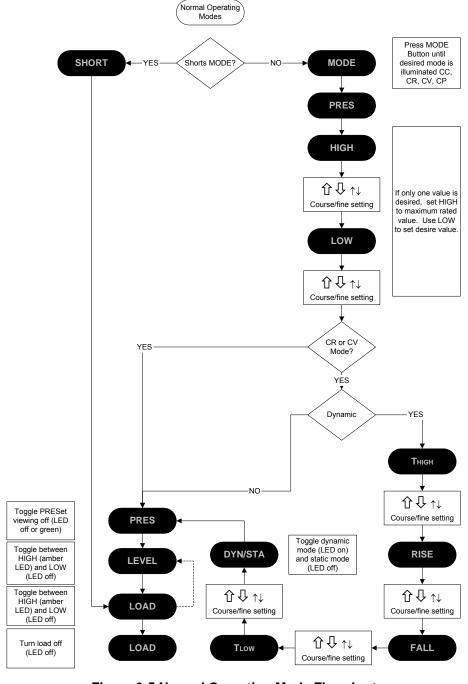
**Figure 3-5 Normal Operating Mode Flowchart**
