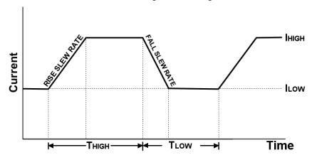
Figure 3-4 Dynamic Mode Waveform and Definition Parameters
