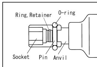
If it is not securely attached, the socket or bit may detach and fly off.
