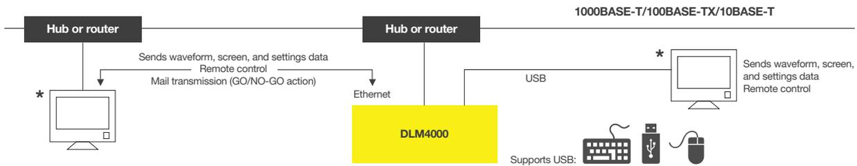
\*DLM4000's internal storage can be recognized by a PC as an external USB storage device. Transferring files is easy even when a USB thumb drive can't be used.
