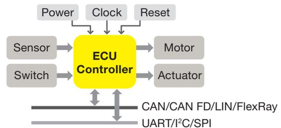
Example: Analog I/O and serial bus controller signals
