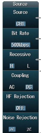
Set the trigger source (CH1 to CH8).
