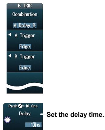
After the trigger A conditions are met and the specified amount of time (the delay time) elapses, the DLM4000 triggers when the trigger B conditions are met.
