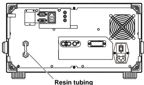
The recommended purge gas flow rate into the AQ6376 is 15 to 20 SCFH (7 to 9.5 L/min).
