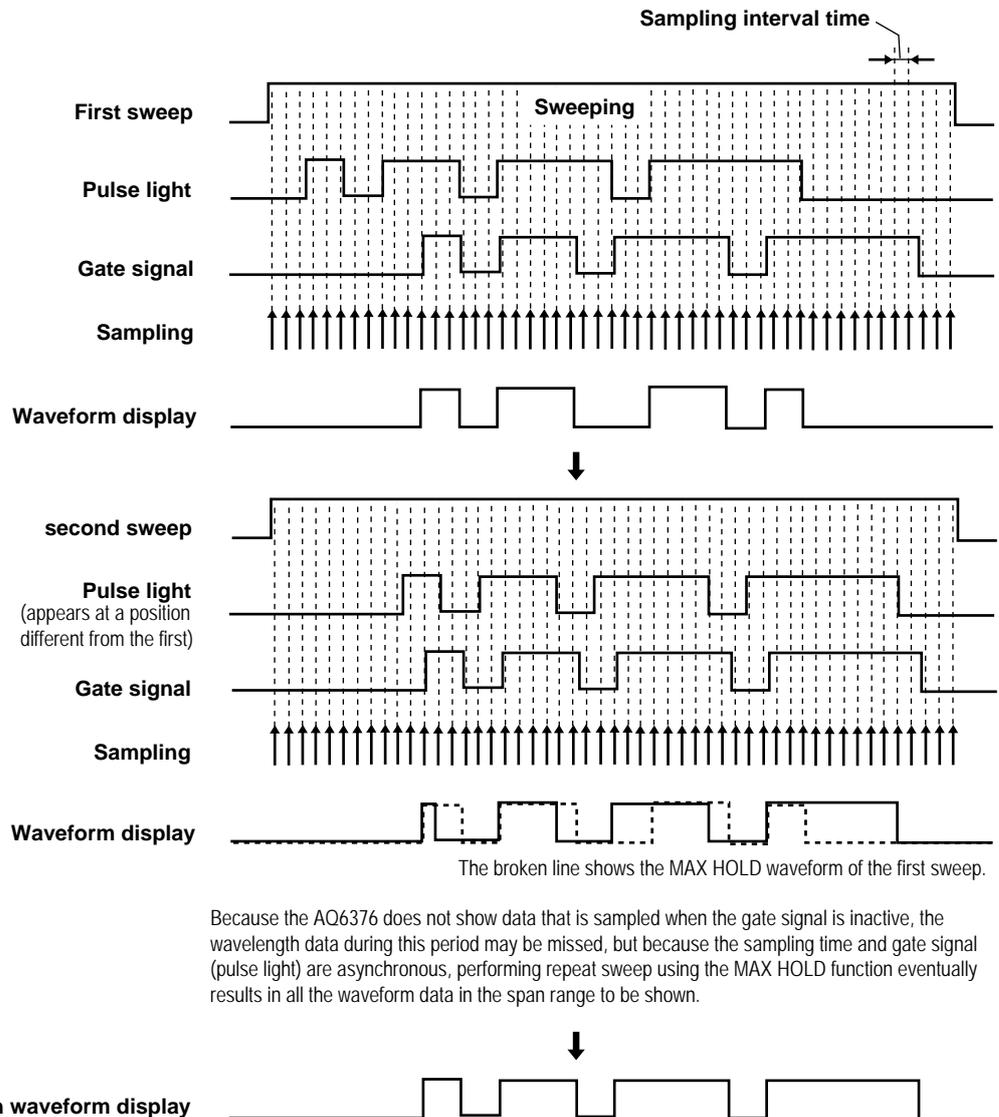
The broken line shows the MAX HOLD waveform of the first sweep.
