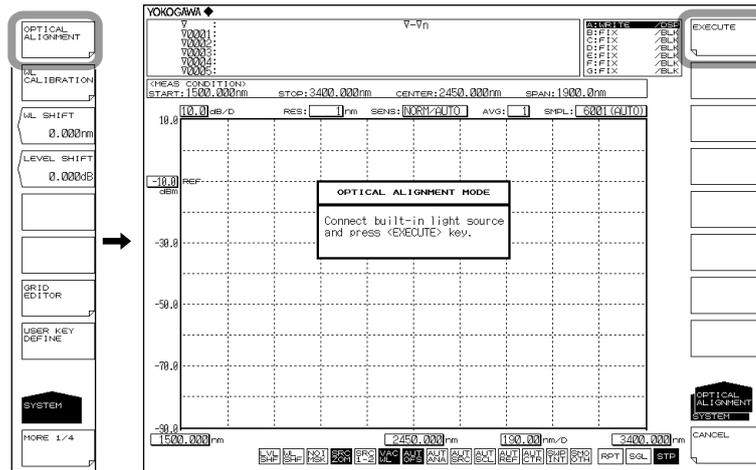
5. Press the **EXECUTE** soft key. Alignment adjustment is automatically executed. Adjustment finishes a few minutes thereafter, and you are returned to the original screen.
