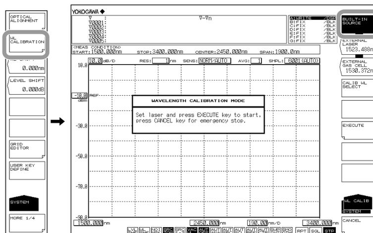
5. Press the **BUILT-IN SOURCE** soft key.
