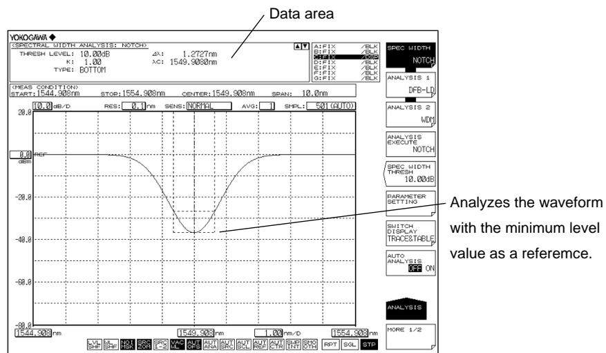
Notch width measured waveform (PEAK)
