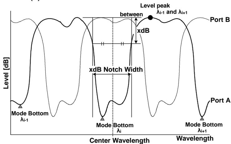
Obtain the width (xdB\_Notch\_Width) between the two points, which are below the higher point of either the left peak level or the right peak level of each channel by the parameter THRESH\_LEVEL, and its center wavelength/frequency (Center\_Wavelength).
