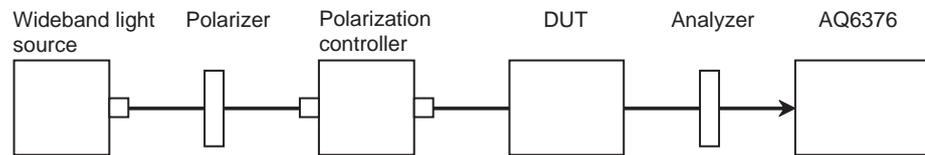
1. Enter measurement conditions so that the entire wavelength range of the wideband light source is measured. Set the resolution to about 0.1 nm.
