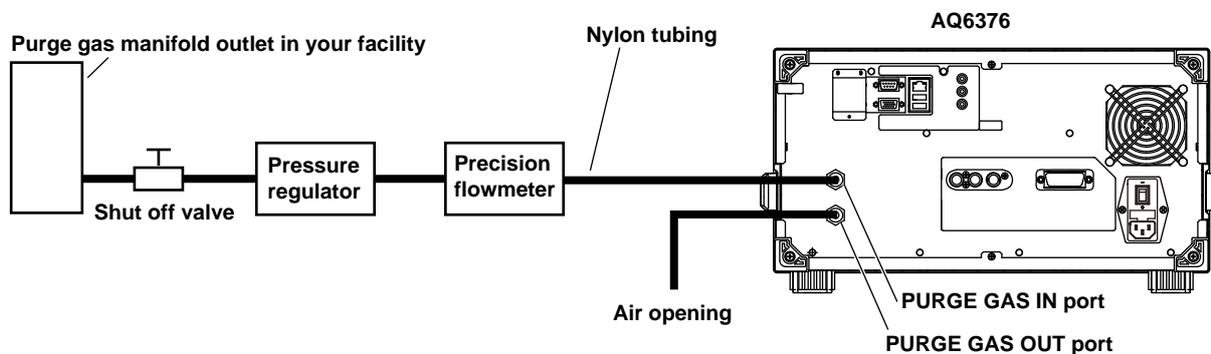
1. Open the purge gas shut off valve then adjust the pressure regulator to provide an appropriate supply pressure below the maximum rating of the precision flowmeter.
