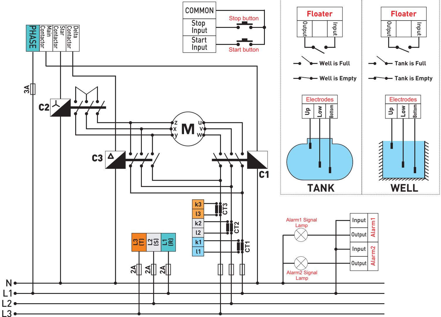
**Note:** To control the level of liquid in the well by electrodes, make connections according to figure 1. Connect floater to the tank. Adjust Pr.34 to 0.
