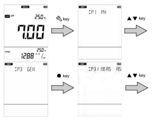
3. Press the ▲ ▼ keys to select "RESET" (initialize) and then press the ● key.
