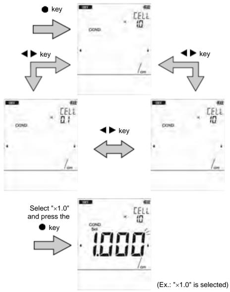
5. Press the ▲ ▼ ◀ ▶ keys to enter the cell constant value of the conductivity cell and then press the ● key to confirm.
