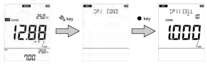
4. Press the ◀ ► keys to select the digit number of the cell constant of the conductivity cell and then press the ● key.
