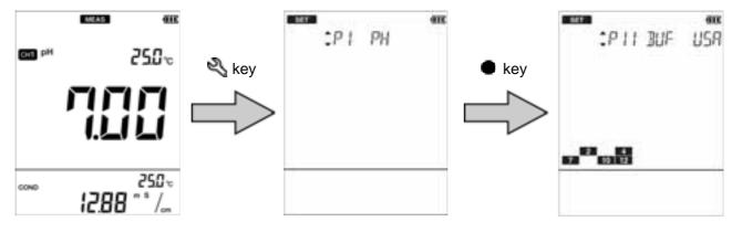
4. Press the ◀▶ keys to select "USA", "NIST", or "CUST" according to the standard solution to be used and then press the ♠ key to confirm selection.
