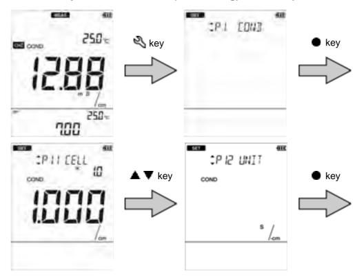
4. Press the ◀ ▶ keys to select the unit and press the ● key to confirm selection.
