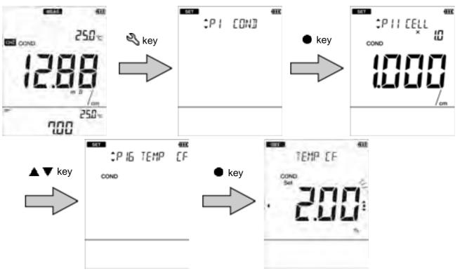
4. Press the ▲ ▼ ◀► keys to enter the temperature coefficient and then press the key to confirm.
