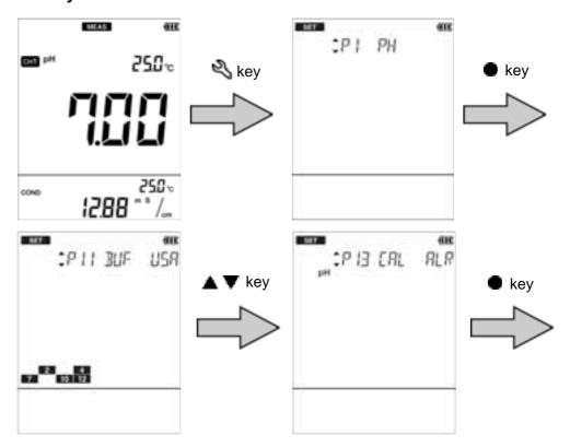
4. Enter the setting period of the calibration interval alarm and then press the key.
