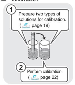
In the following cases, perform conditioning of the electrode before calibration.
