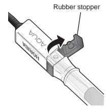
Fill the internal solution with a dropper.
