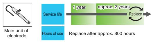
Replace consumables at the period whichever occurs first; approx. two years after purchase or after approx. 800 hours of use, depending on sample solution, measurement frequency, and measurement environment
