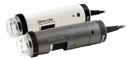
Featuring with FLC and AMR, the Dino-Lite Edge 1.3MP AF4515ZT was made to be tool of choice for measurement-intensive applications within 20-220X magnification. With the adaptable interface which supports the connection to WF-20, a Wi-Fi streamer, the AF4515ZT could be transformed into a wireless microscope on an as-needed basis.
