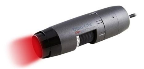
The AM4115T-DFRW Dino-Lite Edge series digital microscope features superior optics, a wide magnification range (20x~220x), and 620 nm (orange) excitation light with a 650nm emission filter for observing deep red fluorescence in subject samples.
