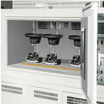
KTE-300 / Durability Tester in Steering wheel and horn Operating
