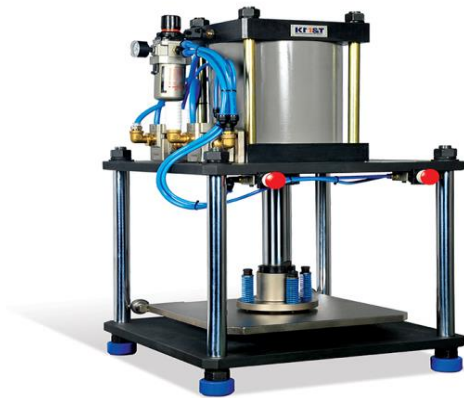
KSCM-1 / Special Cutting Machine / Preparing Specimens
