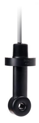
The Sensorex TCS series toroidal (inductive) conductivity sensors feature wide measurement ranges and dependable toroidal technology over the range 0-2000 ms/cm. Resistant to corrosion, coatings, and fouling common to contacting conductivity sensors, the TCS series is designed for a long and trouble-free service life.
