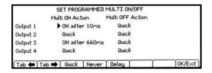
Delay sets a time value in milliseconds between 10ms and 20,000ms (20 seconds)
