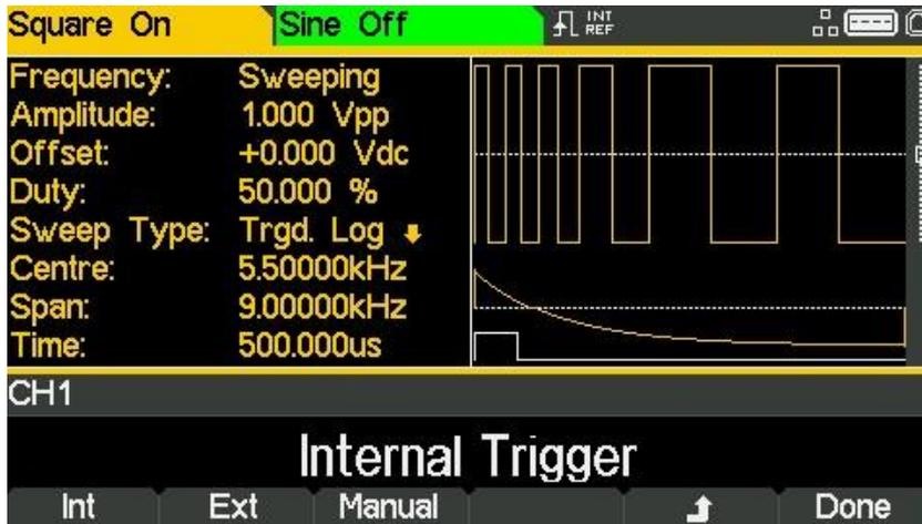
Select the trigger source then press
