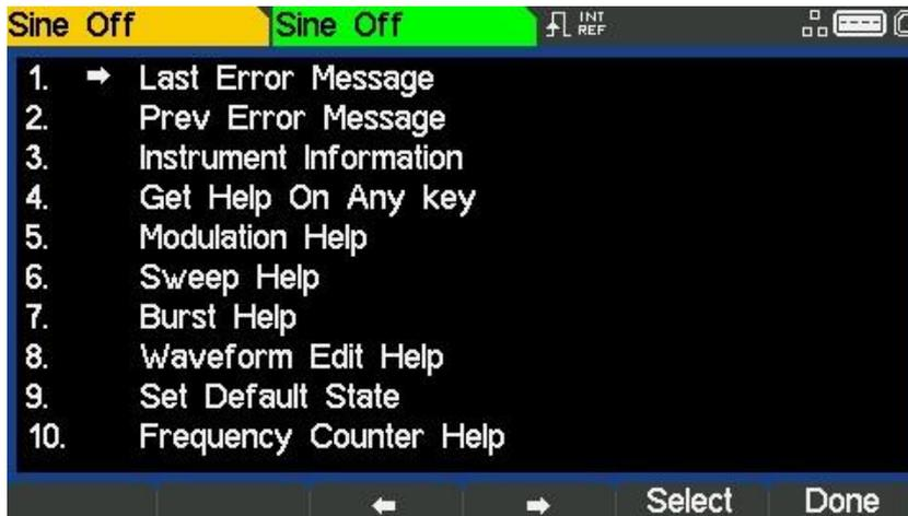
The Help menu uses all the screen space between the Status Line and the Soft-key Labels and contains a list of help topics. To show a topic use the **←** and **→** soft-keys to move the highlight back or forward through the list to select the required topic, then press the **Select** soft-key to show the topic screen.
