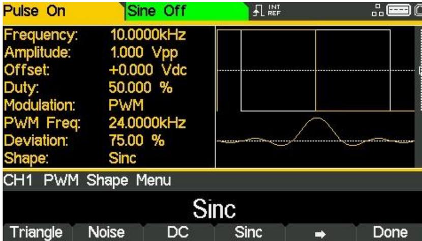
Select the modulation shape required by pressing the appropriate key then press the **Done** soft-key to return to the top-level modulation menu.
