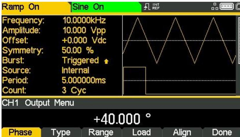
The carrier waveform in the Graph Box will show a representation of the carrier start phase as the phase is edited.
