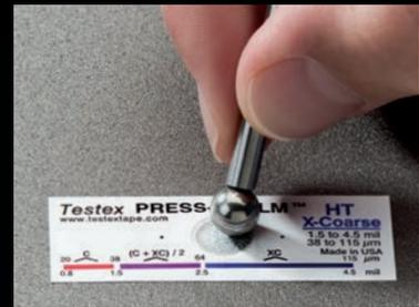
For use with Testex™ Press-0-Film™ Replica Tape
