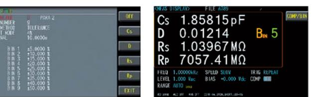
BIN settings for one specific parameter of the selected measurement parameters provide up to 9 BIN positions. Set the judgment basis for individual classifications according to the desired BIN methods (EQUAL/SEQUENTIAL/TOLERANCE/RANDOM) and limit value mode (VALUE/delta/delta%). The result of this sorting can be obtained through the Handler interface. If directly connected to an external device such as a sorter, an immediate sorting can be performed.
