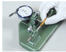
Measurement example for swing of round bar.
