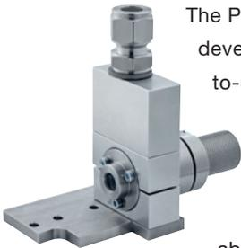
The PCF2.5 cyclone module has been developed to provide a robust, simple-to-use instrument designed to remove coarse particles from the raw gas drawn out of a CVS tunnel. It typically cuts off particles with aerodynamic diameter above 2.5 µm. It is used to fulfill the recommendations according the UNECE R83 and R49 regulations.
