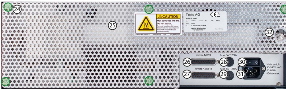
Fig. : rear view of testo ASET15-1 with safety cage mounted
