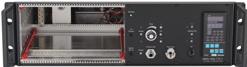
Fig.5.1: testo ASET15-1 without integrated testo MD19-3E Rotating Disk Diluter
