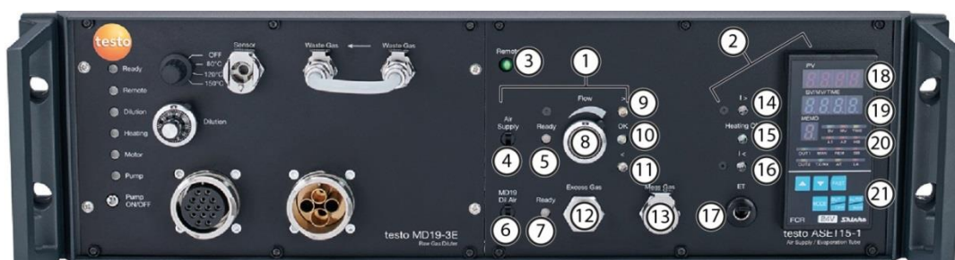
Fig.4.3 : front view of testo ASET15-1 with integrated testo MD19-3E
