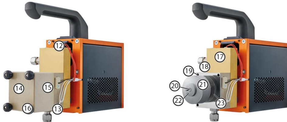
Fig. 4.7: diluter head with removed heat protection hood
