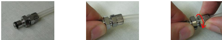
Fig. 5.4: one end of the waste gas bridge with plug
