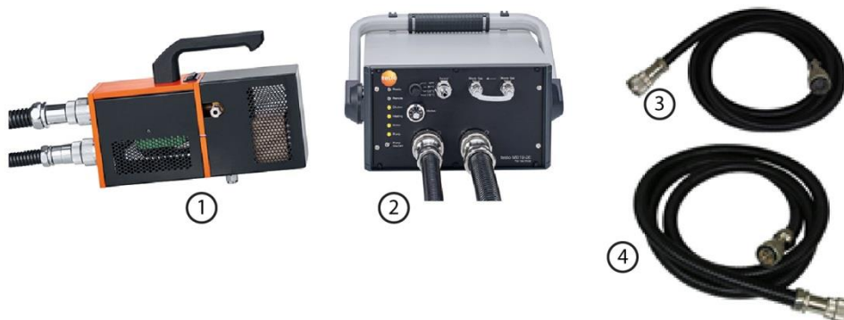
Fig. 4.5: diluter head 1), control unit 2), electrical 3) and pneumatic 4) connections
