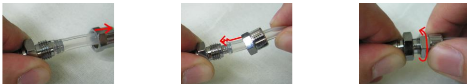
Fig. 5.5: install a different tube
