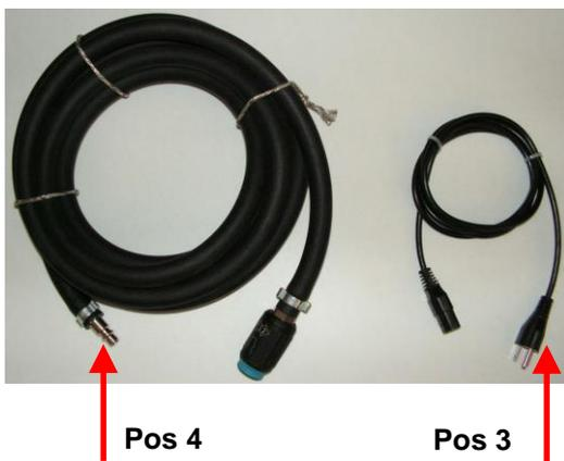
Fig. 5.8: Air hose and power cable
