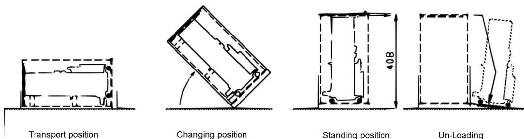
Fig. 5.1: Unpacking testo REXS
