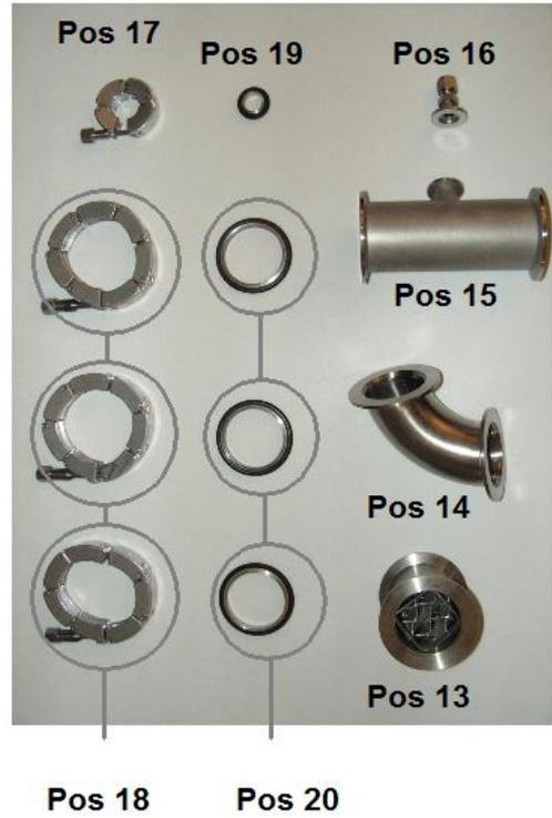
Fig. 5.7: Flanges, centering rings and bulkhead rings
