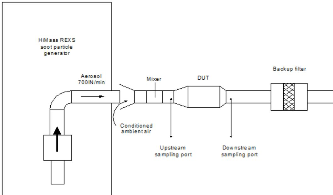
Fig. 6.4: The DUT is not directly connected to the aerosol output. In this measuring configuration the aerosol flow is diluted by conditioned ambient air
