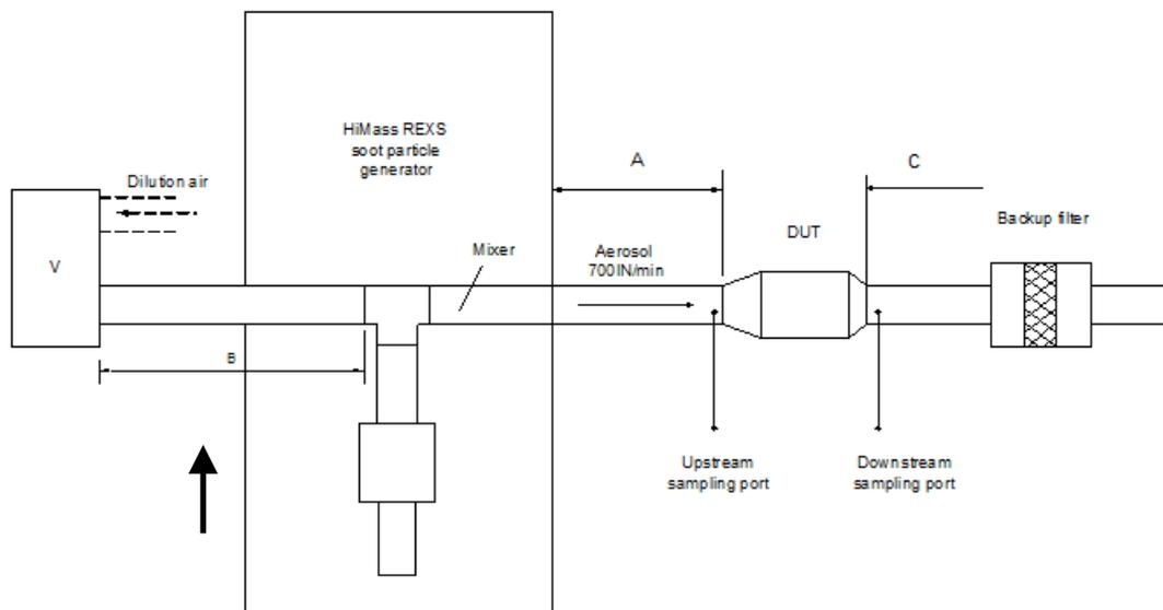
Fig. 6.3: Direct connection of the testo REXS to the DUT with additional dilution air supply with volume (V) to avoid pulsation
