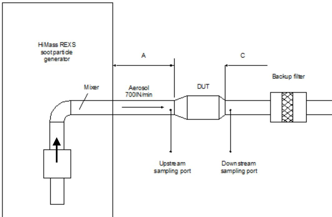
Fig. 6.1: Direct connection of the testo REXS to the DUT
