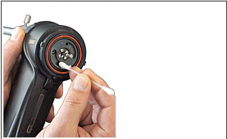
6. Clean the stator disc using a moistened cotton bud and rub dry with an unused cotton bud.
