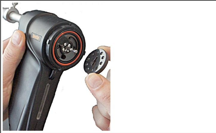
7. Replace the rotation disc (pay attention to the locking pin on the particulate matter probe and the protrusion on the rotation disc).
