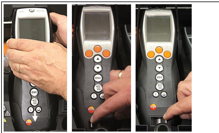
3. Insert the testo 330 into the holder and fix in place using the locking lever.
