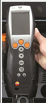
2. Lift up the repository for the testo 330 and insert the measuring instrument.
