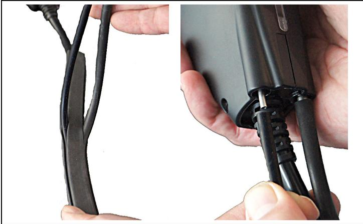
3. Insert new crude gas and/or measurement gas tube. Please ensure that the hose is inserted into the protective cover correctly. Connect crude gas and/or measurement gas tube to the particulate matter probe.
