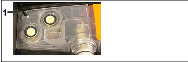
1. Place cover cap (1) on the fresh air inlet of the condensate container.
