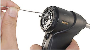
5. Insert the brushless side of the cleaning brush into the gas path
