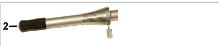
3. Place cover cap (2) on the probe shaft of the particulate matter probe.
