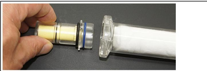
4. Remove the primary filter from the cotton filter.
