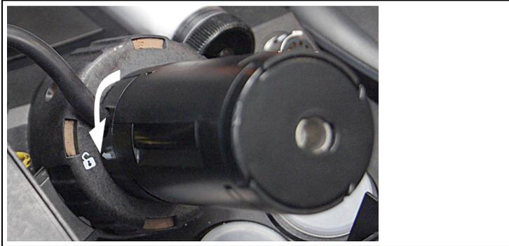
2. Unlock the preheating section (anti-clockwise) and remove.
