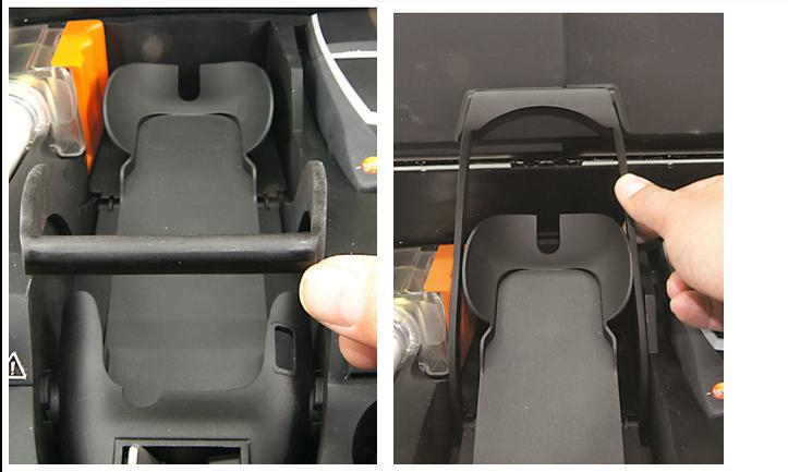
1. Fold up securing clip and click into place on the case lid.
