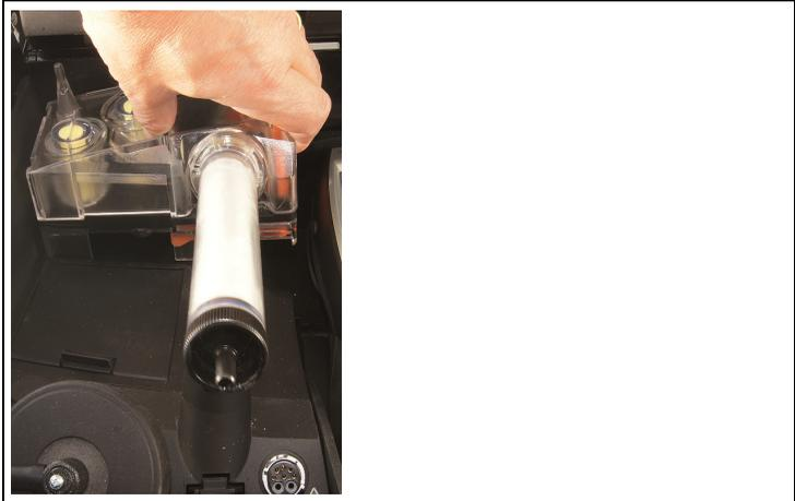
2. Remove condensate container horizontally from the testo 380.
