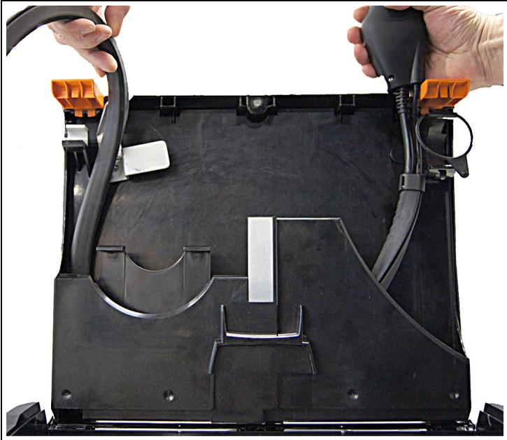
5. Put probe cable into the storage compartment.
