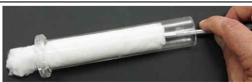
6. Remove the cotton from the filter chamber.
