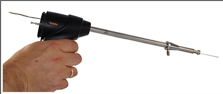
6. Push the cleaning brush through to the probe shaft tip.
