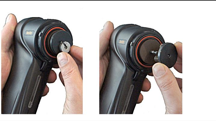
3. Depress the lock and pressure element and remove the lock. Then remove the pressure element via the shaft.
