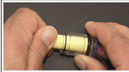
6. Remove the exhausted filter and replace it with a new one.
