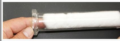
9. Fill the filter chamber evenly with 5 g new cotton wool. Do not compress cotton wool unnecessarily.
