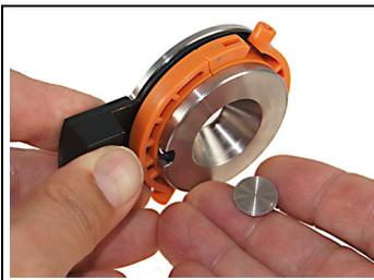
7. Carefully remove the nozzle from the nozzle pot. Avoid touching the nozzle area.
