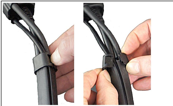
1. Open sealing clip and remove from the protective cover.
