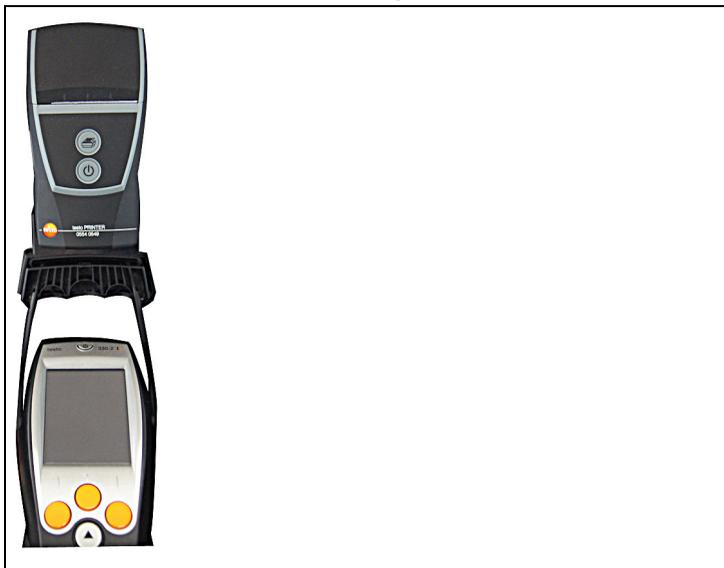
To transfer data from the measurement system to the IrDA record printer, the printer is attached to the magnetic plate (on the top of the testo 330).
