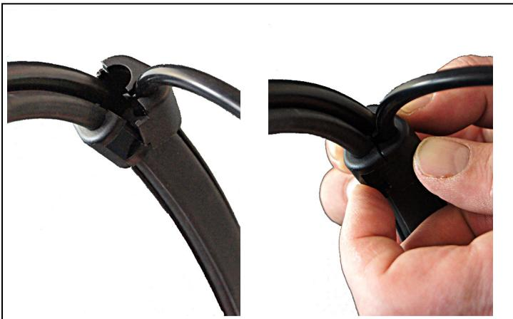
4. Insert crude gas and/or measurement gas tube each into one half of the sealing clip and carefully push the halves together (audible click).
