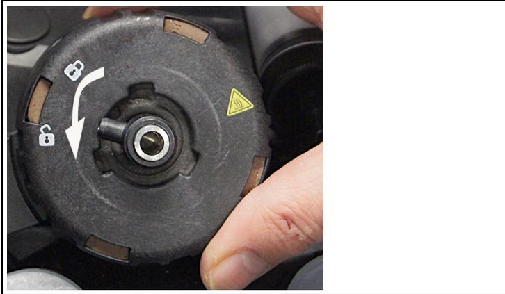
4. Unscrew the particulate matter sensor cover (anti-clockwise) and remove.
