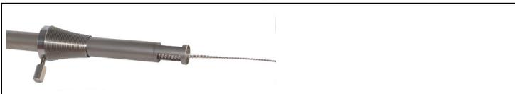
7. Pull the cleaning brush out of the probe shaft. Repeat steps 5 and 6 several times depending on the degree of contamination.
