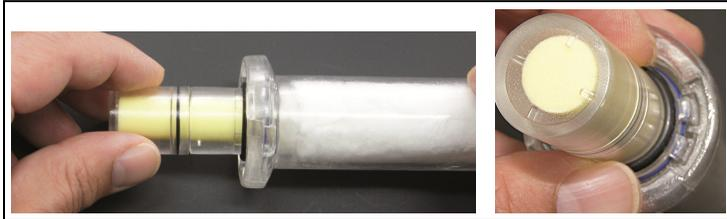
7. Close the primary filter housing, place back on the cotton filter and press into position. Pay attention to the notch on the primary filter.
