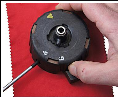
6. Push down on the orange markings with a suitable tool and remove the cover.
