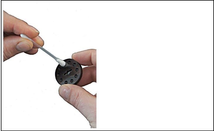
**i** Use distilled water to clean the rotation and stator disc.
