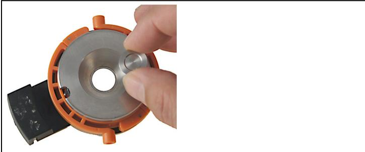
1. Carefully insert nozzle into the nozzle pot (the side with the inscription facing downwards).
