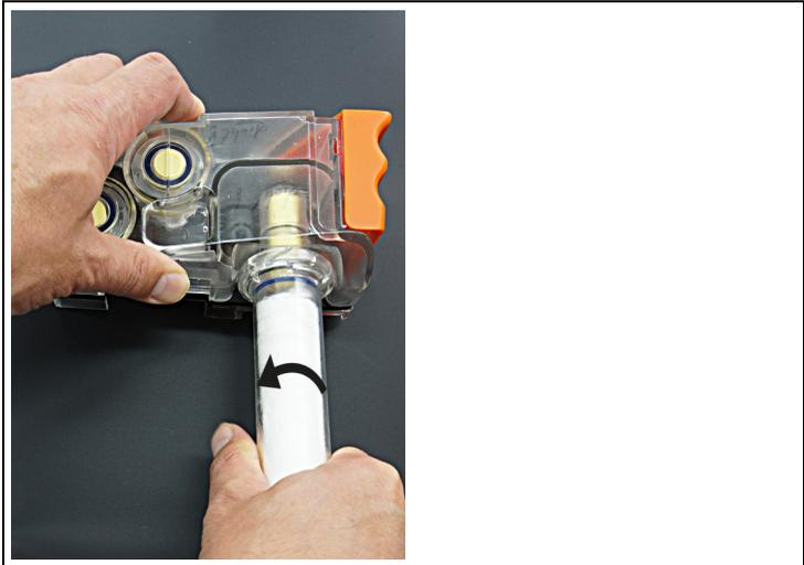
3. Unscrew the cotton filter (anti-clockwise) and remove.
