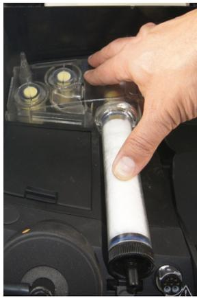
6. Insert the condensate container into the testo 380 and click into place. Push the tube onto the connector.
