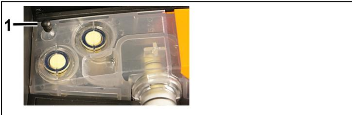
2. Place cover cap (1) on the fresh air inlet of the condensate container.
