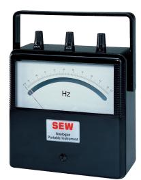
The Hz meters use a frequency-to-DC current transducer which drives a high sensitivity moving coil type indicator. It features accurate frequency measurements without noticeable influence of line voltage fluctuation (50 to 300V) or waveform distortion.
