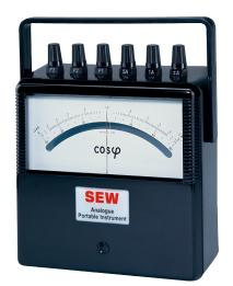
The PF meter is used for measurement in single-phase and balanced threephase circuits. From a phase discriminating circuits, the output of the builtin transducer produces a DC proportional to the phase between voltage and current to operate the DC indicator.
