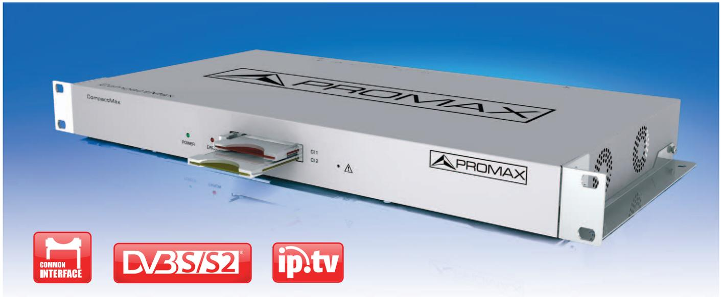
**CompactMax-5** is a compact transmodulation system that allows to distribute Satellite TV channels (DVB-S or DVB-S2) in IPTV format (TS over IP). It can be connected to up to **4 satellite inputs** (2 inputs for free channels and 2 for encrypted ones) to deliver up to 10 IPTV streams (SPTS or MPTS) with dynamic webserver management via remote control. It is integrated into a 19" 1U Rackmount case. It can also be mounted directly on the wall.
