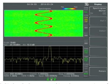
**Figure 64.** Displays both spectrographic and spectrum views of the signal.
