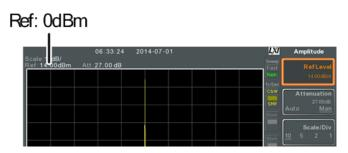
**Figure 28.** Before reference level offset(offset: 0dB)
