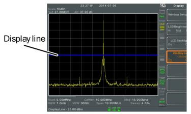
Figure 60. Display line set at -50 dBm
