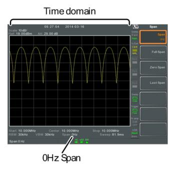
Figure 23. Example: Amplitude modulation
