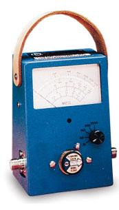
The **IC-002** (81050) directional wattmeter is an accurate, portable, RF power meter using a Rotary Detection Component to measure Direct and Reflected Power in 5 selectable power ranges. Model 81050 includes "Quick Match" type connectors for greater versatility. The instrument is delivered with a carrying case containing compartments for loads and connectors.
