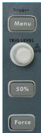
Figure 13. Trigger Control Zone.
