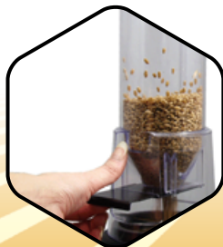
2. Empty loader into analyzer
