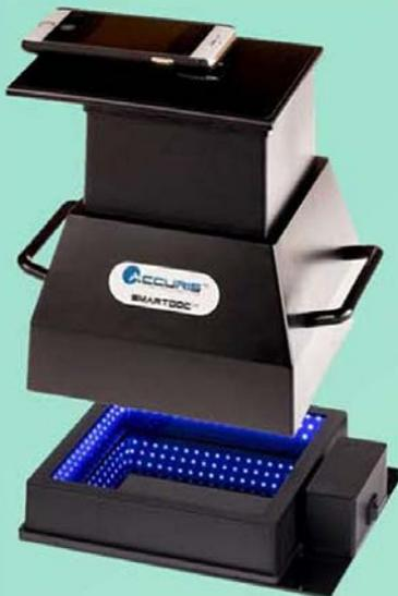
**Imaging enclosure fits over the blue light illumination base**
