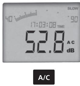
After switching on the device, correspondingly switch over the dB A/ dB C weighting filter by pressing the "A/C" button.
