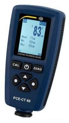
Combined Coating thickness tester for capture of the thickness of coating, plastic.../ measuring of steal/iron (F) and non-ferrous objects (NF) / single or permanent measurement
