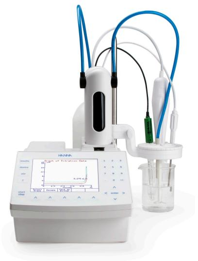
This new generation of titrator features a 50% smaller footprint for maximum use of your lab space. The sealed body is precision-engineered to resist spills and dust and a high-contrast display shows you everything you need to know during testing.
